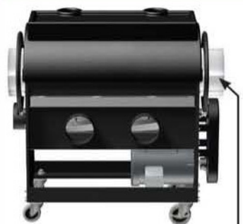
Note the longer end of the TUMBLER when re-installing
